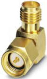
Adapter, SMA (female) -> SMA (male), right-angle; insertion attenuation <0.3 dB at 2.4 GHz
