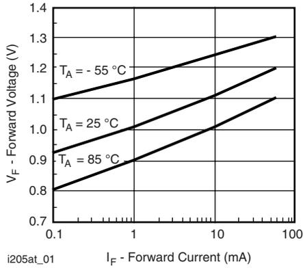
Fig. 1 - Forward Voltage vs. Forward Current
