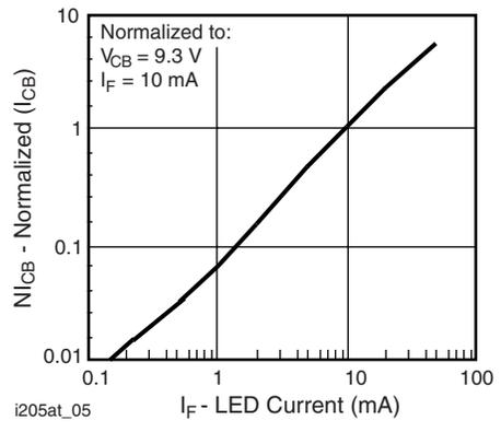
Fig. 5 - Normalized Collector-Base Photocurrent vs. LED Current
