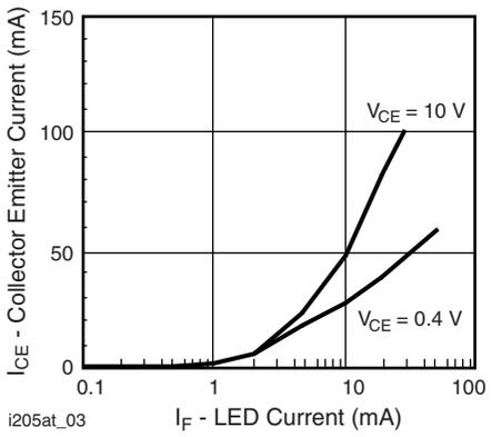
Fig. 3 - Collector Emitter Current vs. LED Current
