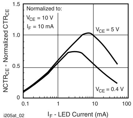
Fig. 2 - Normalized Non-Saturated and Saturated CTR<sub>CE</sub> vs. LED Current
