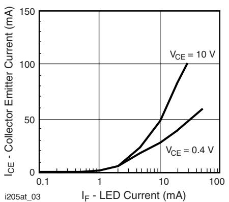
Fig. 3 - Collector Emitter Current vs. LED Current
