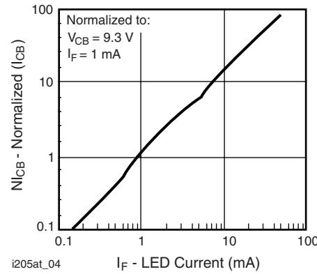
Fig. 4 - Normalized Collector-Base Photocurrent vs. LED Current
