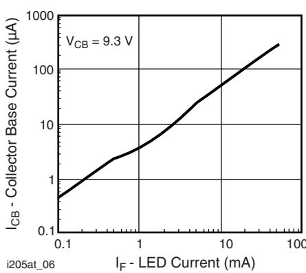
Fig. 6 - Collector Emitter Photocurrent vs. LED Current
