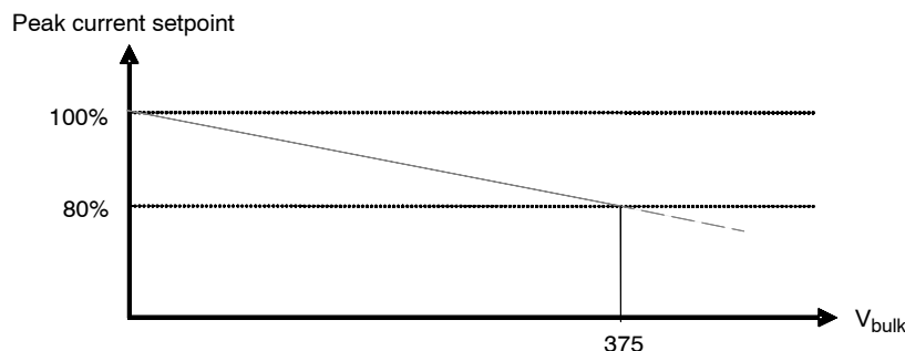
Figure 33. The peak current regularly reduces down to 20% at 375 V dc.
