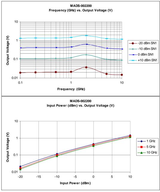
The MADS-002200 in an SC-79 Package Style was evaluated in a detector circuit in which the Schottky diode terminates a 50 Ohm transmission line on a duroid substrate. The SC-79 packaged diode was attached to the terminal of a 3.5mm connector and the output voltage was measured through a bias tee on a voltmeter. Matching was not attempted.
