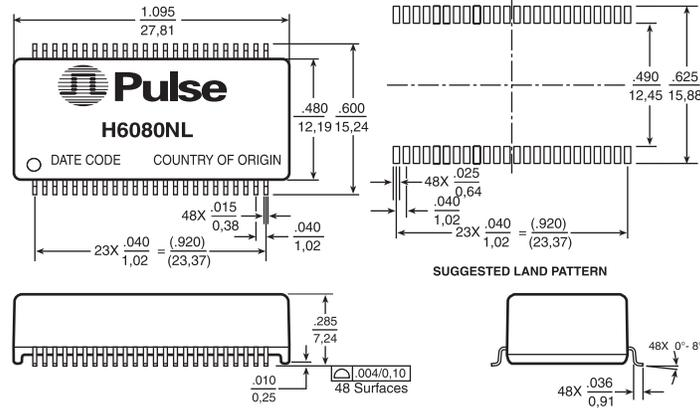
Dimensions:  $\frac{\text{Inches}}{\text{mm}}$  Unless otherwise specified, all tolerances are  $\pm \frac{.010}{0,25}$
