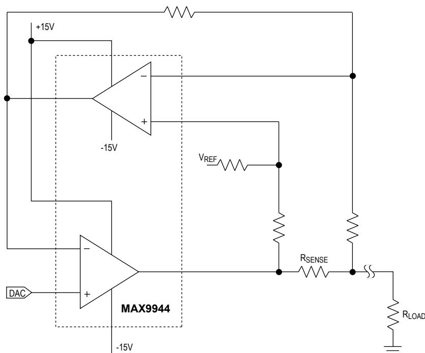
*Figure 3. Typical  $\pm 20\text{mA}$  Current-Source in Loop-Powered Systems*
