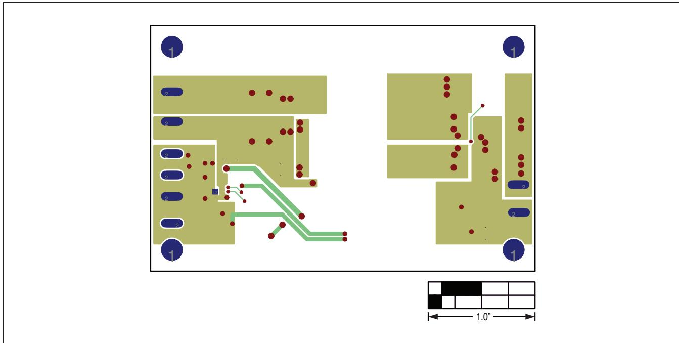
Figure 8. MAX17598 EV Kit PCB Layout—Solder Side
