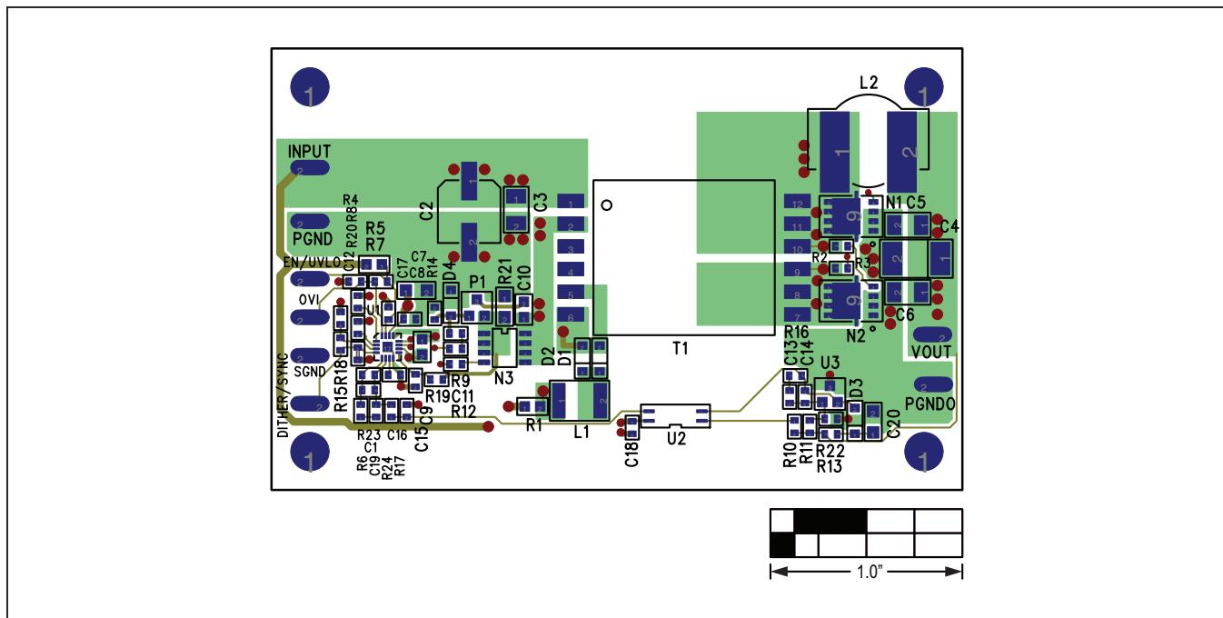
Figure 7. MAX17598 EV Kit PCB Layout—Component Side
