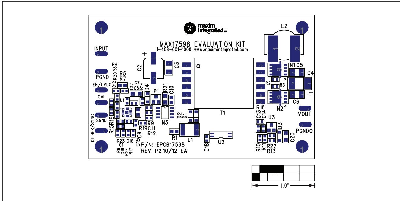
Figure 6. MAX17598 EV Kit Component Placement Guide—Component Side
