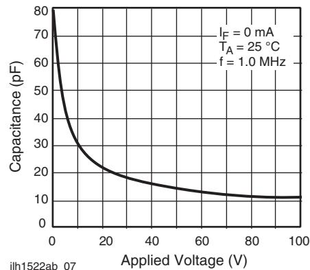
Fig. 8 - Switch Capacitance vs. Applied Voltage
