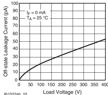
Fig. 11 - Leakage Current vs. Applied Voltage
