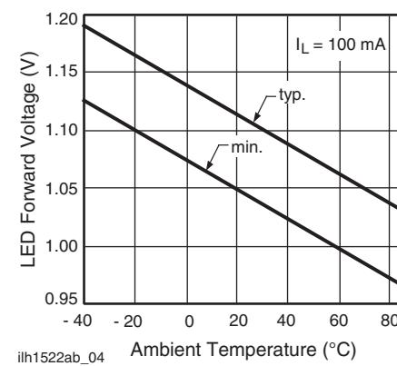
Fig. 5 - LED Dropout Voltage vs. Temperature
