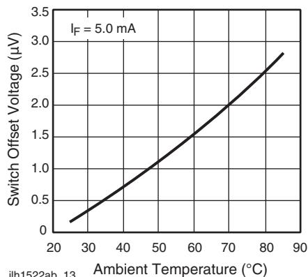
Fig. 14 - Switch Offset Voltage vs. Temperature
