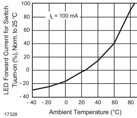
Fig. 3 - LED Current for Switch Turn-on vs. Temperature
