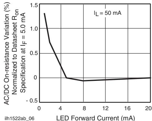
Fig. 7 - Variation in On-Resistance vs. LED Current
