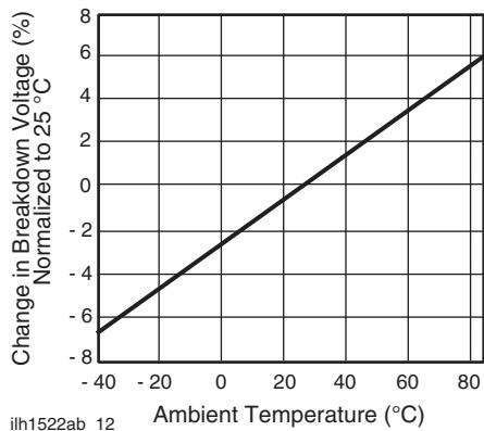
Fig. 13 - Switch Breakdown Voltage vs. Temperature
