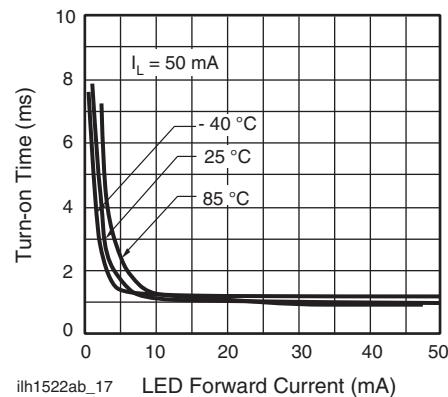
Fig. 18 - Turn-on Time vs. LED Current
