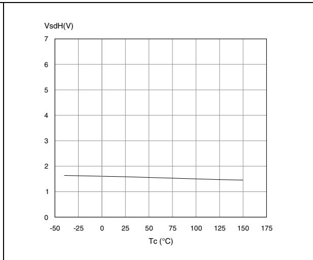
**Figure 31. Low level STAT\_DIS voltage**
