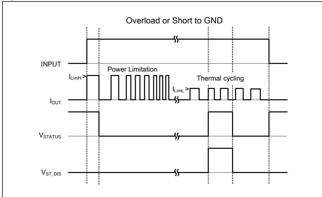
**Figure 10. Intermittent overload**
