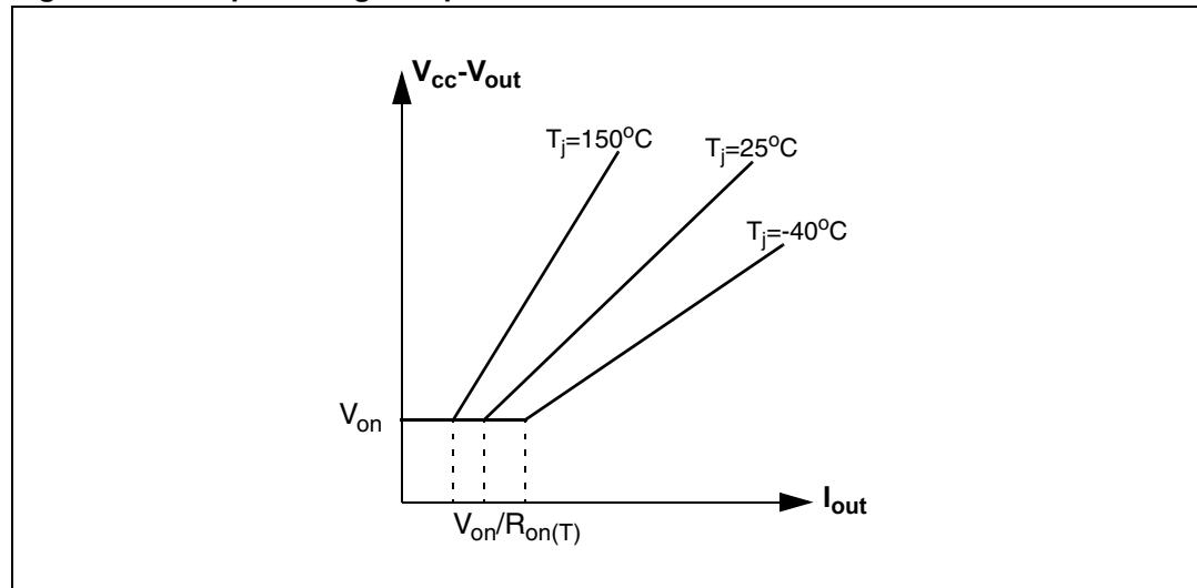
**Figure 6. Switching characteristics**
