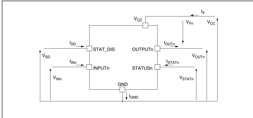
1.  $V_{Fn} = V_{OUTn} - V_{CC}$  during reverse battery condition.
