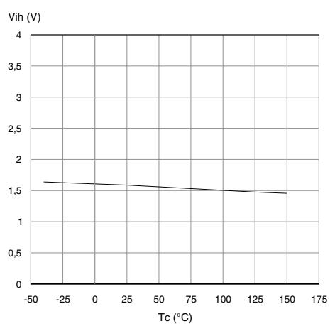
Figure 19. Input low level voltage
