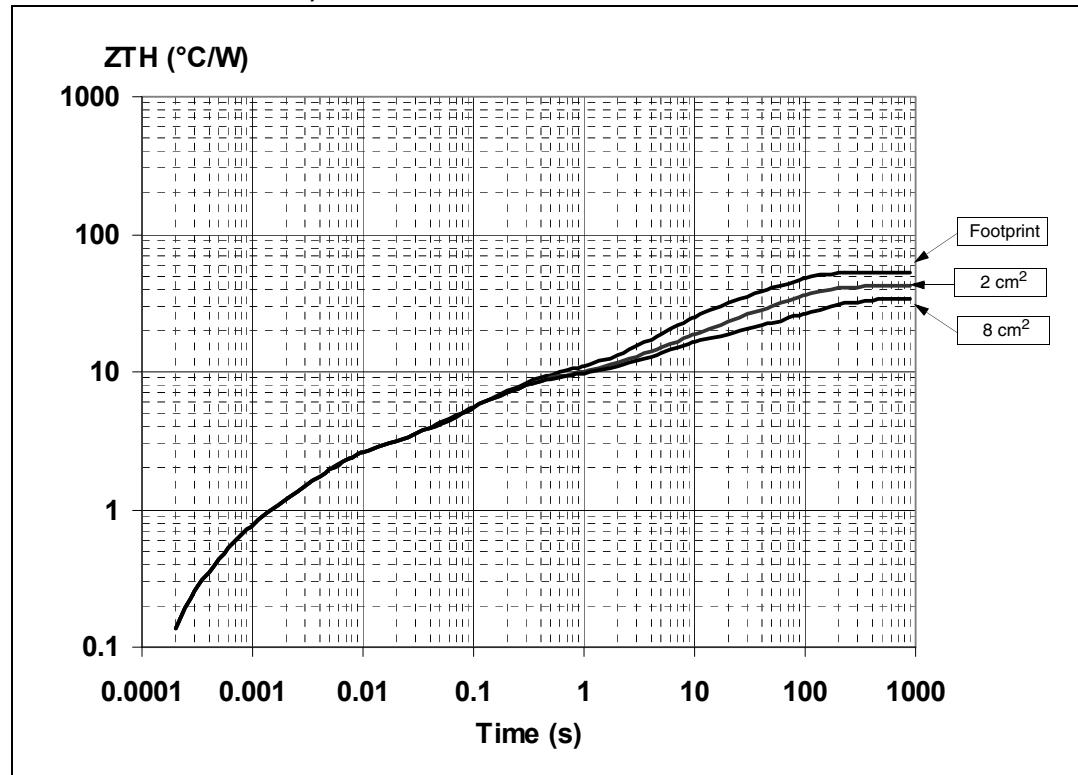
**Figure 38.** Thermal fitting model of a double channel HSD in PowerSSO-24<sup>(1)</sup>
