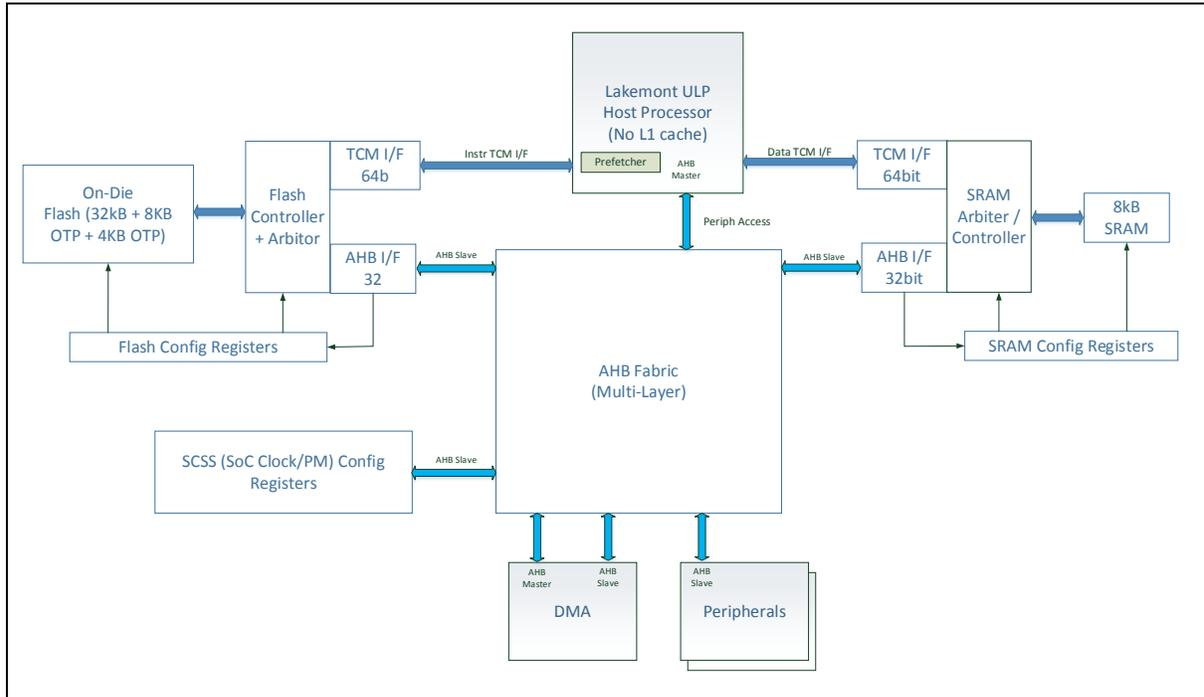
From memory consistency analysis perspective, Intel® Quark™ microcontroller D2000 consists of following key IPs:
