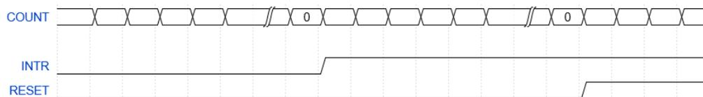
The counter is reloaded by writing 76h to the Counter Restart Register, this will also clear the WDT Interrupt.
