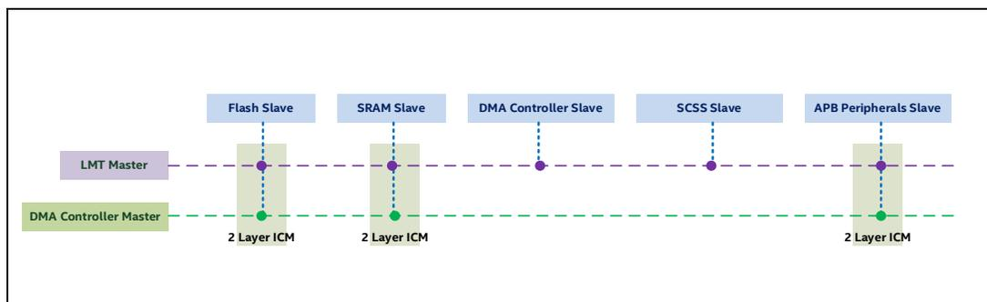
From an address decode perspective, DMA controller can target all destinations inside Flash subsystem (Flash Configuration registers, Instruction Flash, 8KB OTP, 4KB OTP) and all destinations inside SRAM subsystem (SRAM and SRAM Configuration registers).
