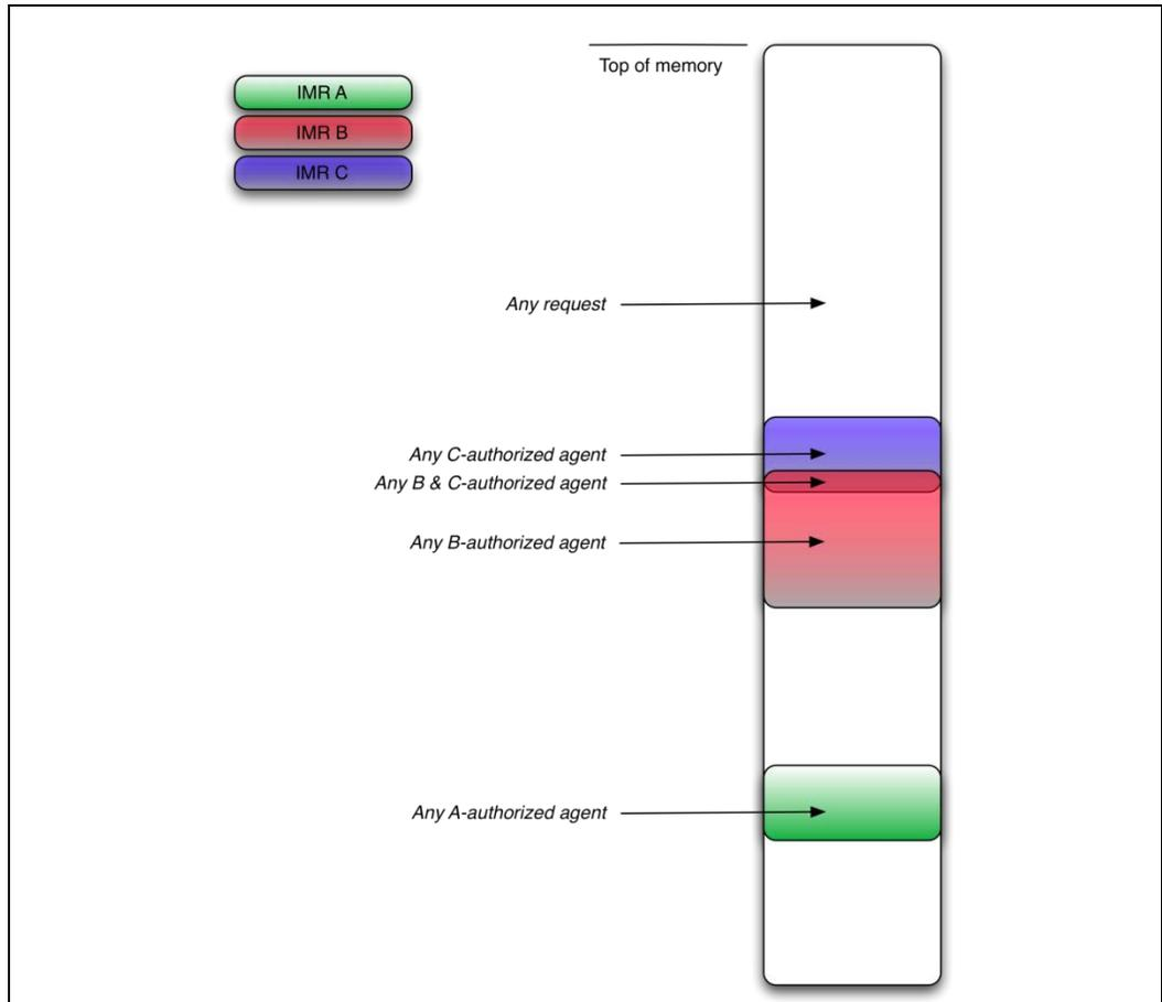
The IMR registers will reside in the SRAM Controller Configuration Registers.
