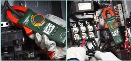
The MA610 is a fully loaded clamp meter with multimeter functions including AC Current, AC/DC Voltage, Resistance, Frequency, and Capacitance. It also has a built-in non-contact voltage (NCV) detector to quickly check circuits and wires for live voltages.
