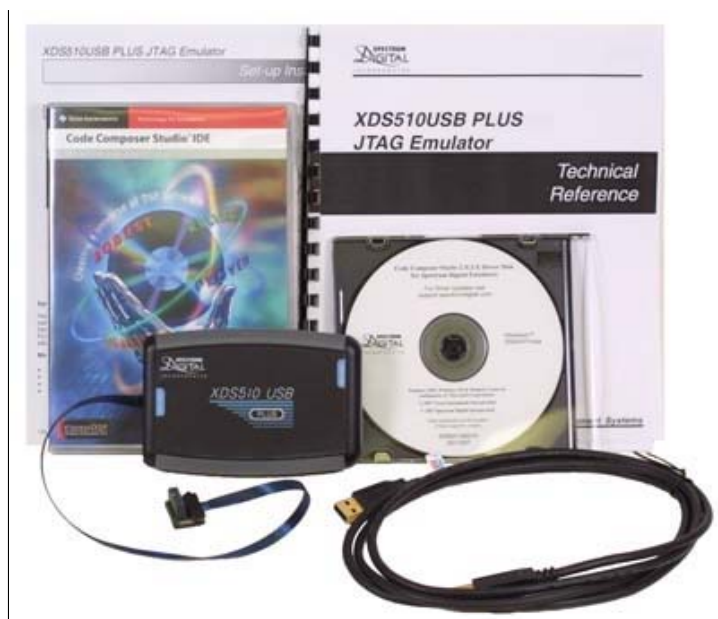
XDS510USB PLUS JTAG Emulator with Code Composer Studio Platinum version 3.3
