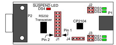
Figure 3. CP2104 Evaluation Board with Default Shorting Blocks Installed
