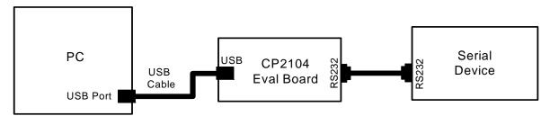
Figure 1. Hardware Setup
