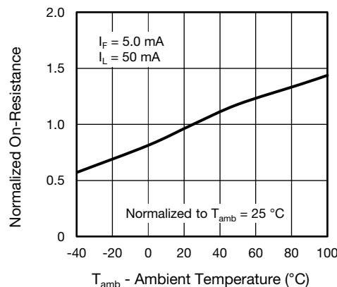
Fig. 9 - Normalized On-Resistance vs. Ambient Temperature
