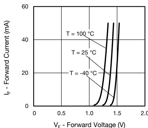
Fig. 7 - Forward Current vs. Forward Voltage
