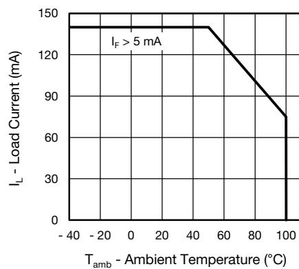
Fig. 5 - Maximum Load Current vs. Ambient Temperature
