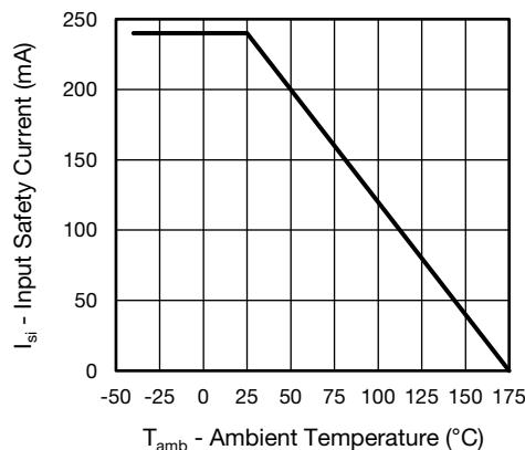
Fig. 4 - Safety Input Current vs. Ambient Temperature
