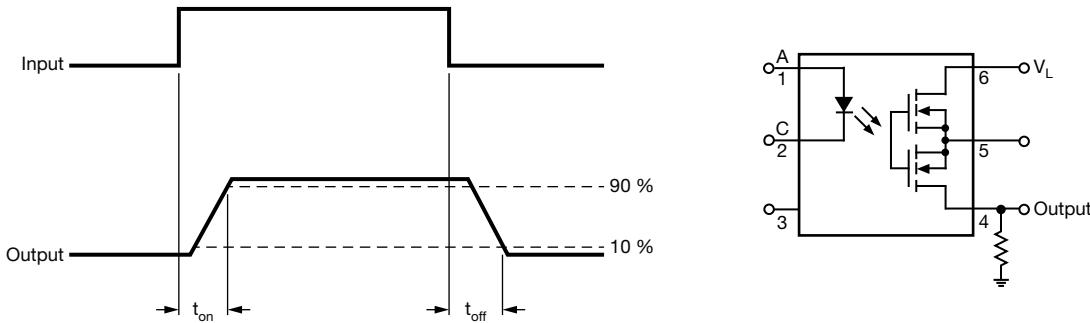
Fig. 2 - Timing Schematic
