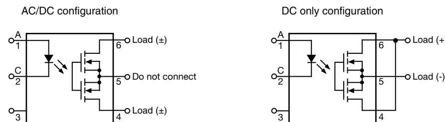
Fig. 1 - Pin Configuration
