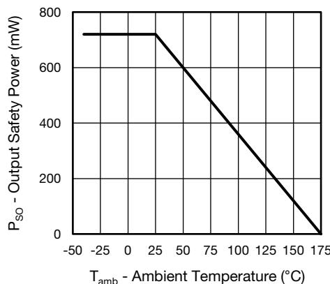
Fig. 3 - Safety Power Dissipation vs. Ambient Temperature
