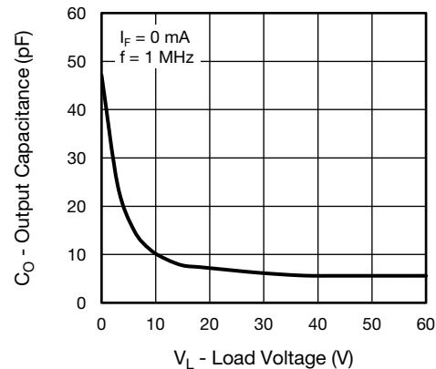
Fig. 10 - Output Capacitance vs. Load Voltage
