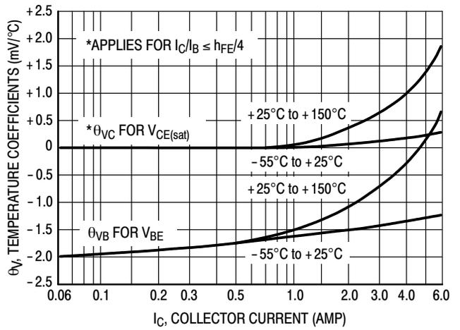
Figure 11. Temperature Coefficients
