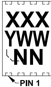
8-Lead DFN (2x3x0.9 mm)
