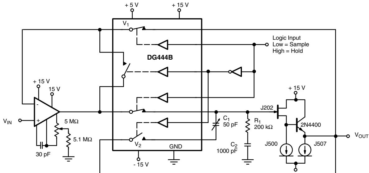
Figure 9. Precision Sample-and-Hold
