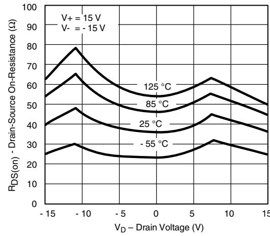
**R<sub>DS(on)</sub> vs. V<sub>D</sub> and Temperature**
