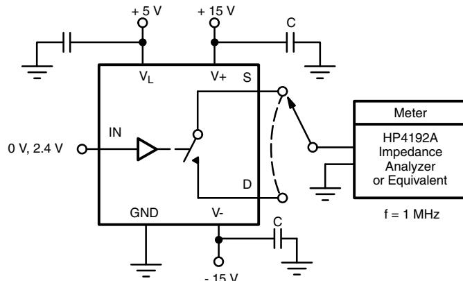
**Figure 6. Source/Drain Capacitances**
