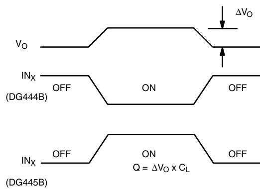
Figure 3. Charge Injection
