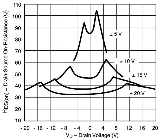
**R<sub>DS(on)</sub> vs. V<sub>D</sub> and Power Supply Voltages**
