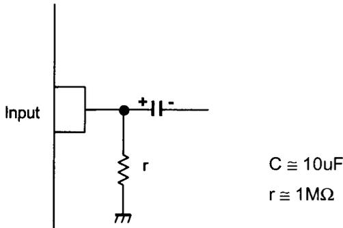
This IC requires  $0.1\mu\text{F}$  capacitor between INPUT and GND,  $1\text{M}\Omega$  resistance between INPUT and GND for clamp type input at mute mode.
