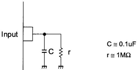
This IC requires  $0.1\mu\text{F}$  capacitor between INPUT and GND for bias type input at mute mode.
