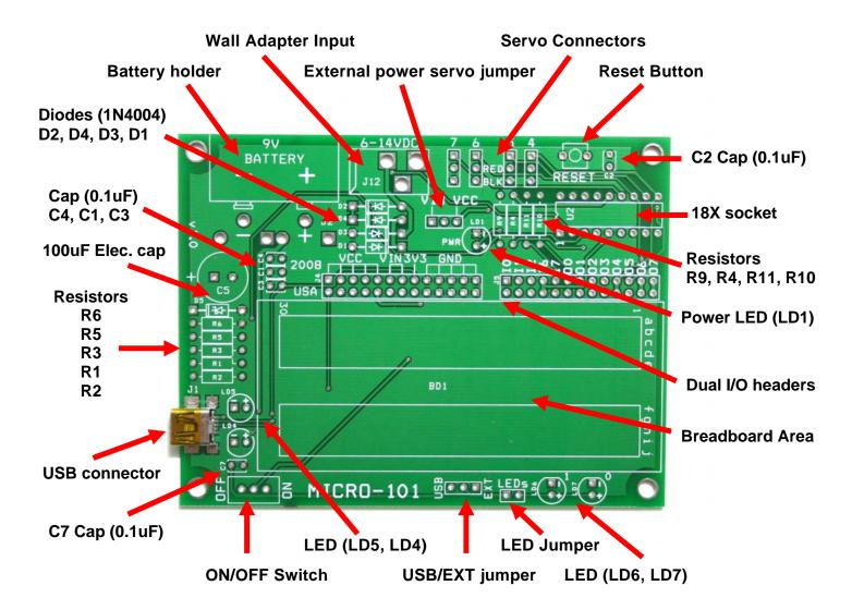
Soldering order is not particularly strict. However, some parts are more difficult to solder than others. Solder the following parts in the order recommended below:
