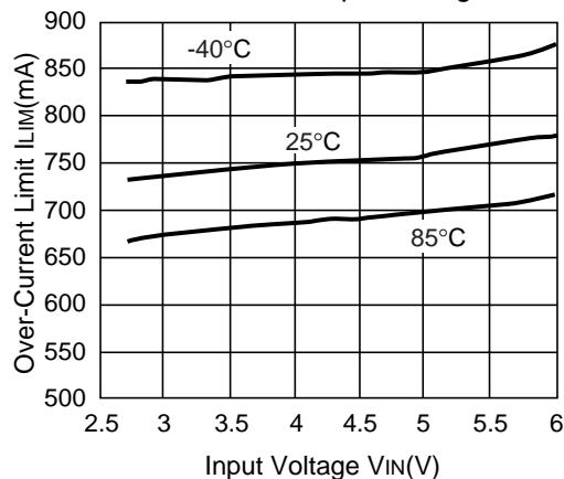
9) Over-current Detector Threshold vs. Temperature
