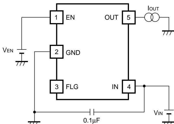
Over-current Threshold Test Circuit
