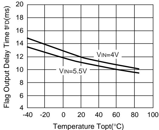
14) Flag Output Delay Time vs. Input Voltage
