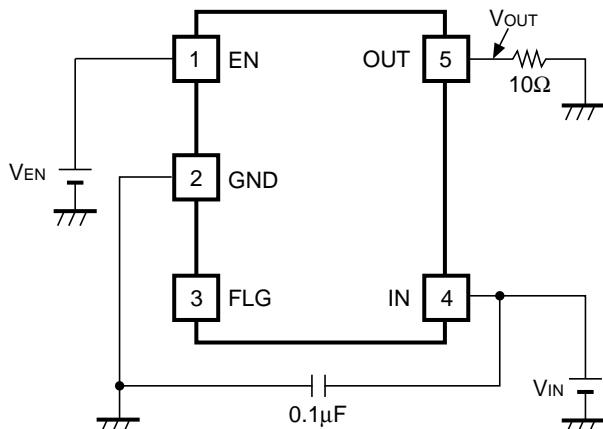
Output On Time Test Circuit
