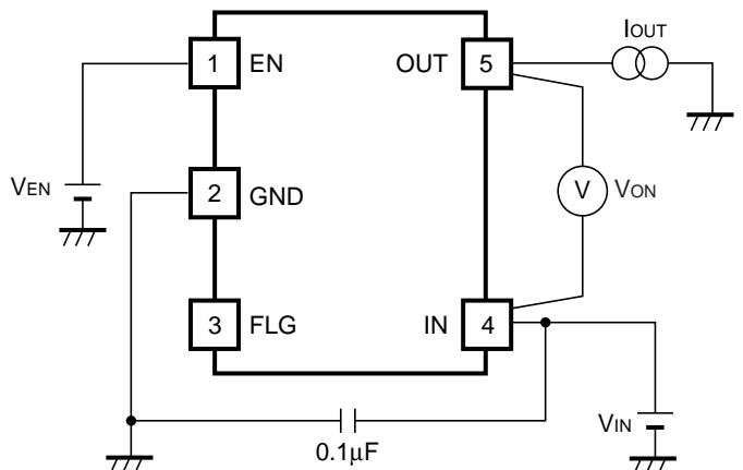
UVLO Threshold Test Circuit
