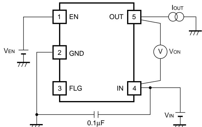
Switch On Resistance Test Circuit
