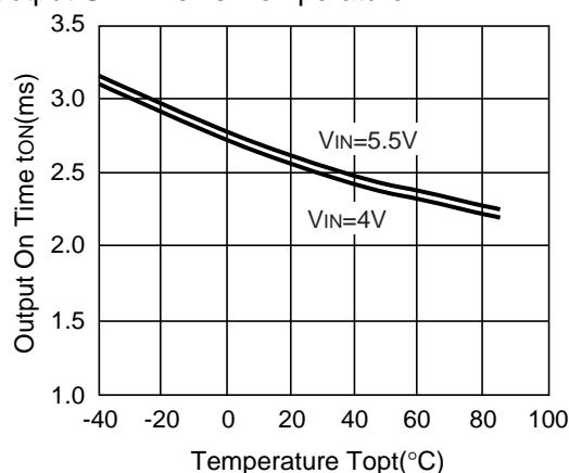
6) Output On Time vs. Input Voltage
