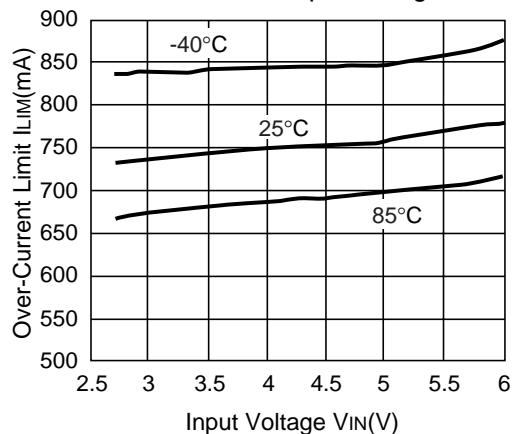
9) Over-current Detector Threshold vs. Temperature
