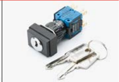
Keylock switch, 3 position, raised, snap-action, rectangular, black plastic, 18x24 mm
