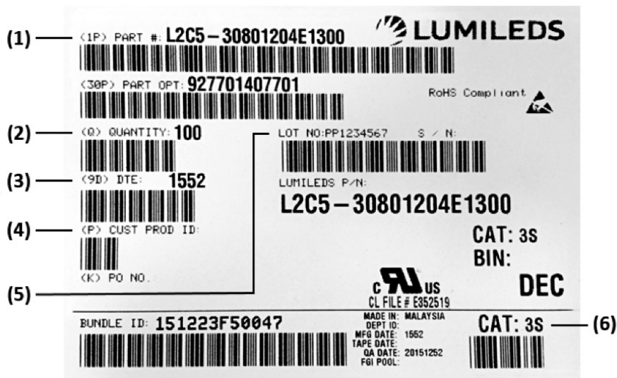
Figure 12. Example of inner box label for LUXEON CoB with CrispWhite Technology (Gen 2).
