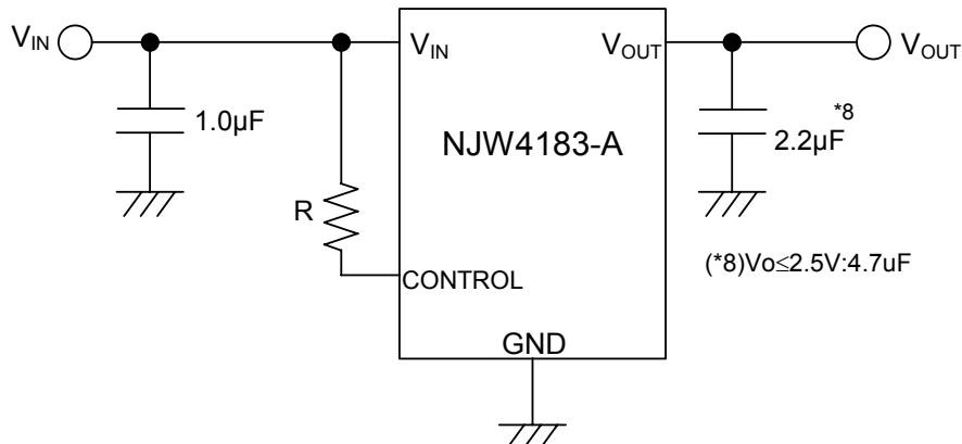
Connect control pin to  $V_{IN}$  pin
