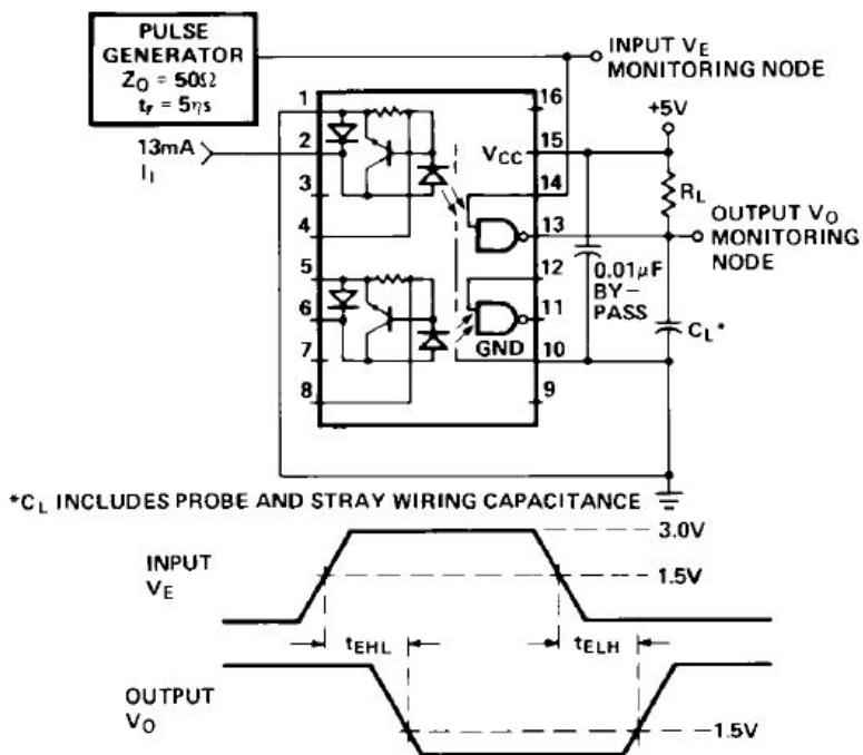
Figure 7. Test Circuit for  $t_{EHL}$  and  $t_{ELH}$ .
