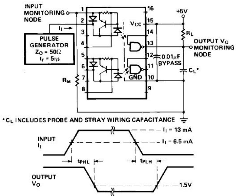
Figure 6. Test Circuit for  $t_{PHL}$  and  $t_{PLH}$ .
