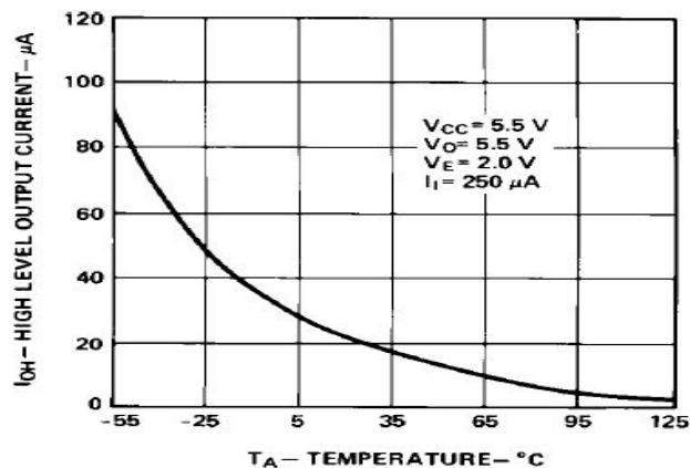
Figure 3. High Level Output Current vs. Temperature.
