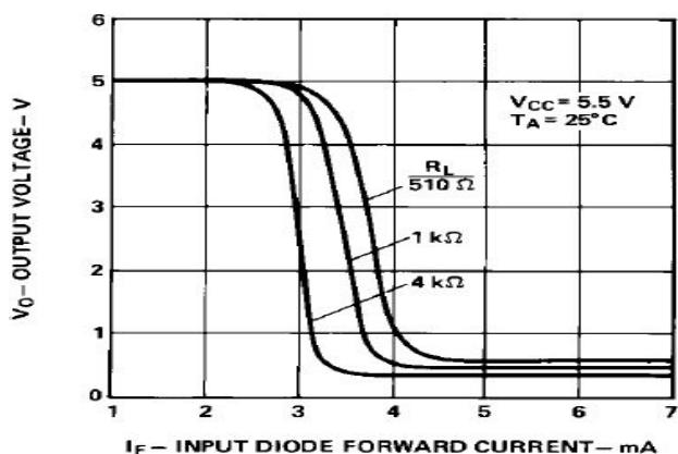
Figure 1. Input-Output Characteristics.
