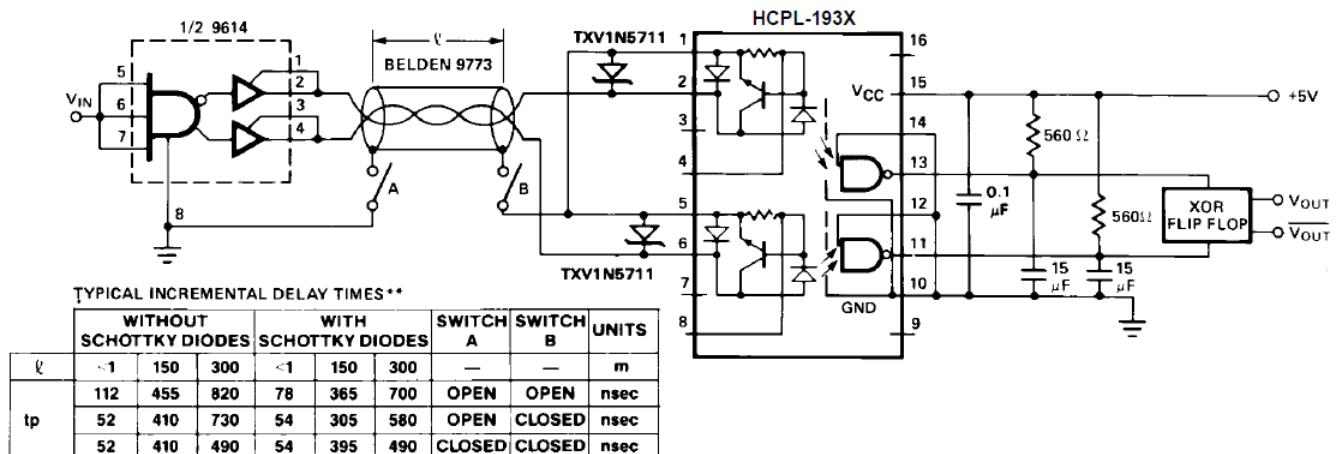
Figure A2. Polarity Reversing, Split Phase.
