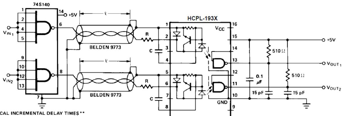
Figure A1. Polarity Non-Reversing.
