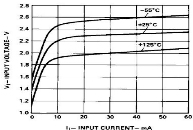
Figure 2. Input Characteristics.
