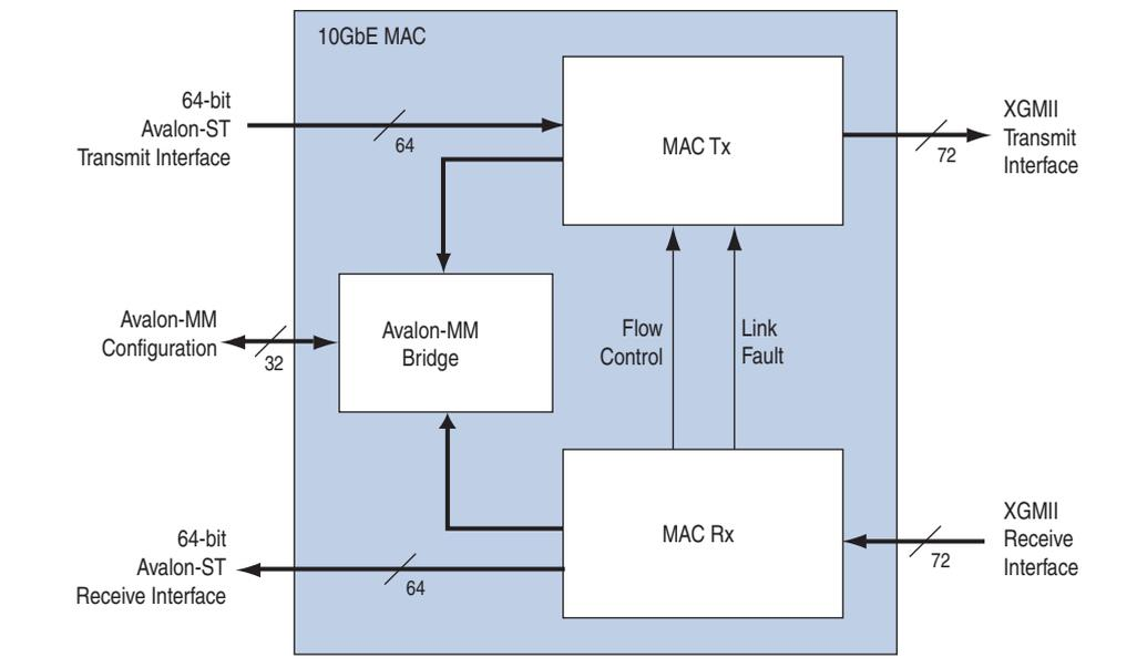
**Figure 7-2. 1G/10GbE MAC IP Core Block Diagram**
