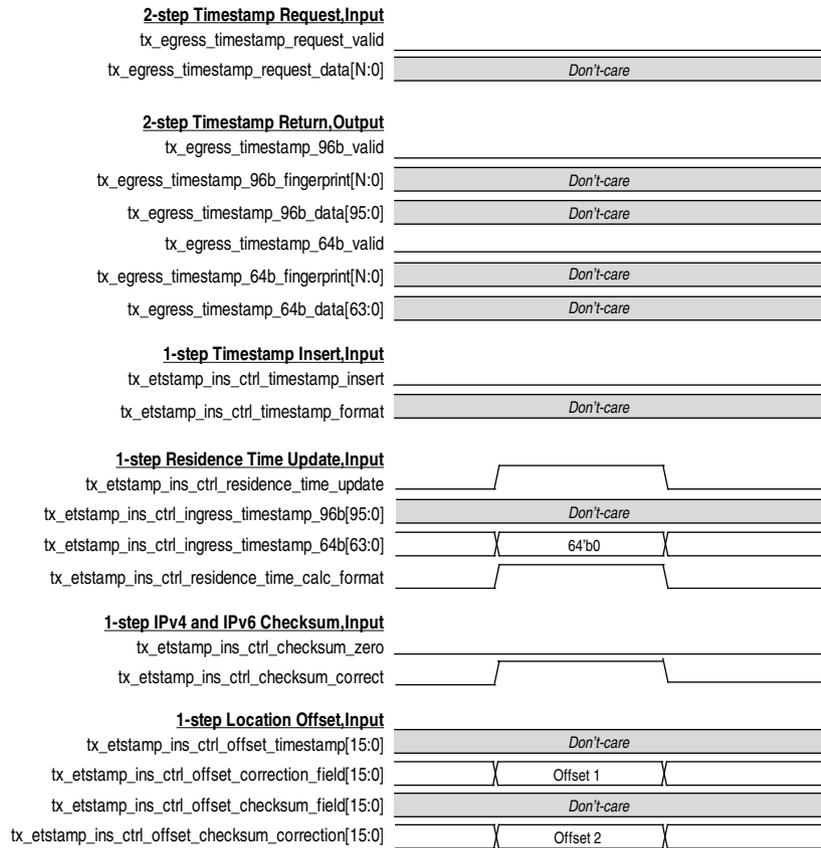
Figure 9-12 shows the TX timestamp signals for the IEEE 1588v2 feature in a two-step operation.
