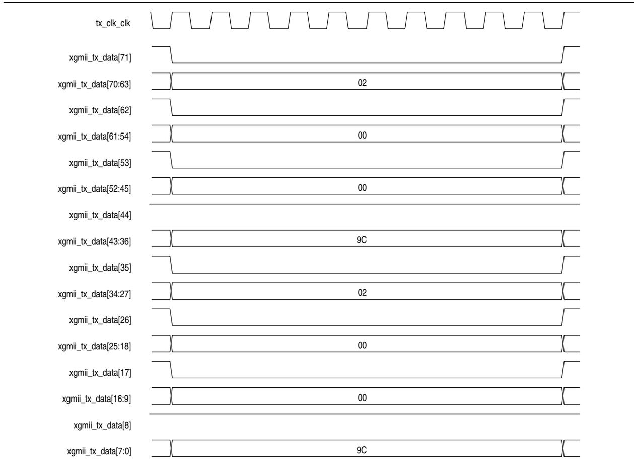
When you instantiate the MAC RX only variation, connect the `link_fault_status_xgmii_rx_data` signal to the corresponding RX client logic to handle the link fault. Similarly, when you instantiate the MAC TX only variation, connect the `link_fault_status_xgmii_tx_data` signal to the corresponding TX client logic. For more information on the signals, refer to “SDR XGMII Signals” on page 9–8.
