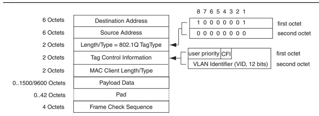
Figure A-3 shows the stacked VLAN frame format.
