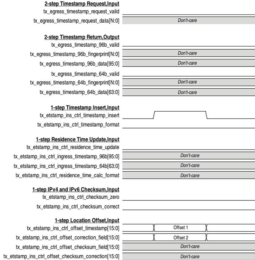
Figure 9-10 shows the TX timestamp signals for the first type of egress correction field update, where the residence time is calculated by subtracting 96 bit ingress timestamp from 96 bit egress timestamp. The result is updated in the correction field of the PTP frame encapsulated over UDP/IPv4.
