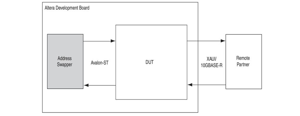
The address swapper swaps the destination address and source address in the receive frame before sending the frame onto the transmit path. You must connect the DUT—design example—to a remote partner that generates, transmits, and receives frames.
