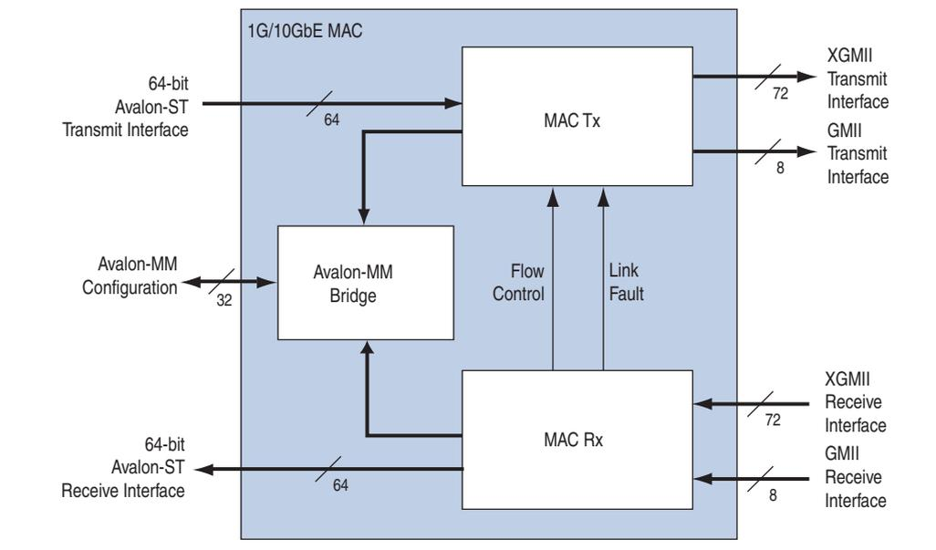
**Figure 7-3. 10M-10GbE MAC IP Core Block Diagram**
