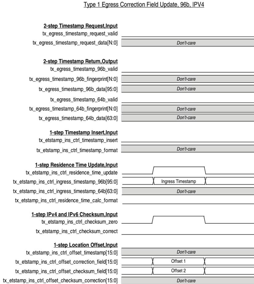
Figure 9–11 shows the TX timestamp signals for the second type of egress correction field update, where the 64 bit ingress timestamp has been pre-subtracted from the correction field at the ingress port. At the egress port, the 64 bit egress timestamp is added into the correction field and the correct residence time is updated in the correction field. This is the example of PTP frame encapsulated over UDP/IPV6.
