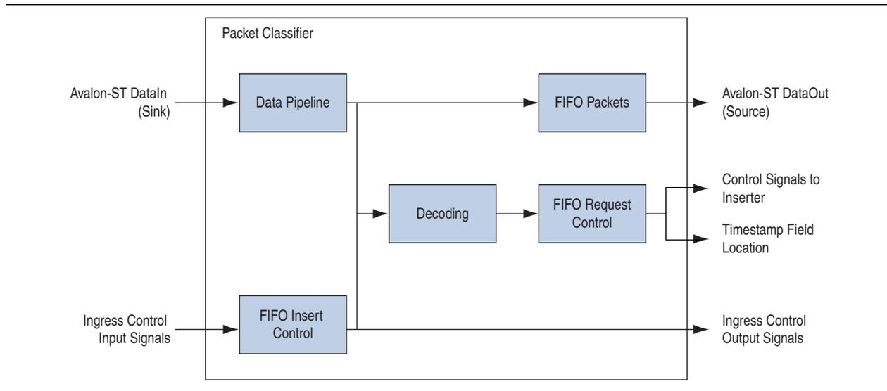
The Packet Classifier block diagram comprises the following components:
