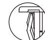
DETAIL VIEW VH1, VH3 & VH5 HOLE PLUGS (No wing serrations for ease of removal)
