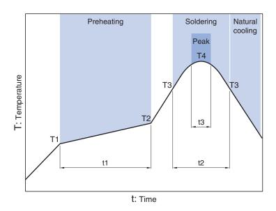
Preheating Soldering Peak Temp. Temp. Time Time Temp. Time T1 T2 T4 Т3 150°C 180°C 120s 230°C 30s 260°C 10s max.
