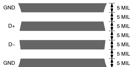
Figure 22. Typical Arrangement of Signal Tracks
