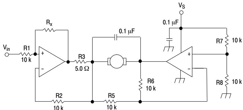
For circuit stability, ensure that  $R_x > \frac{2R_3 \cdot R_1}{R_M}$  where,  $R_M$  = internal resistance of motor.
