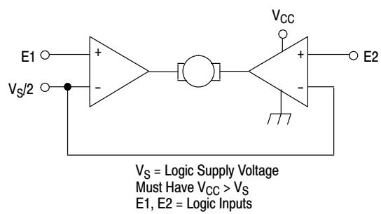
**Figure 9. Bidirectional DC Motor Control with Microprocessor-Compatible Inputs**
