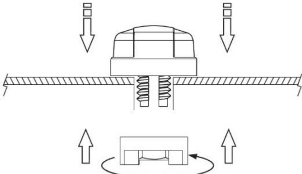
Recommended torque for Mounting is  $24.5\text{N}\cdot\text{m}$
