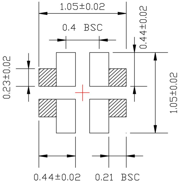
**Disclaimer:** This is only a recommendation based on information available to Micrel from its suppliers. Actual land pattern may have to be significantly different due to various materials and processes used in PCB assembly. Micrel makes no representation or warranty of performance based on the recommended land pattern."
