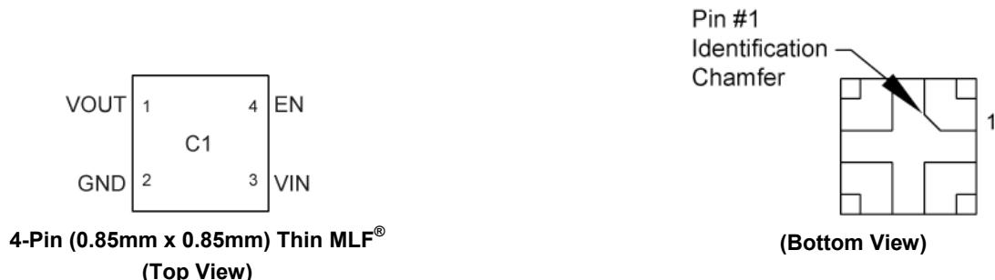
Example Showing Orientation of Part Marking
