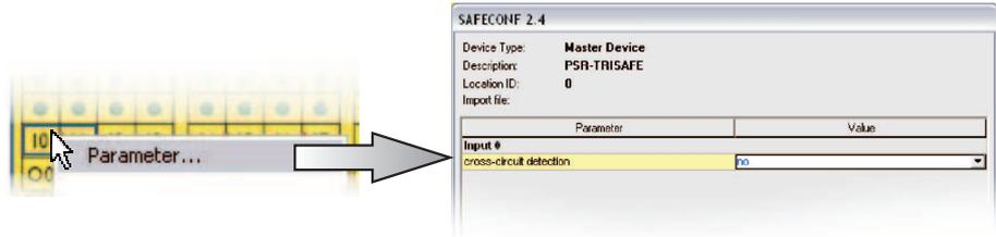
Figure 4-11 Opening the device parameterization editor via the context menu
