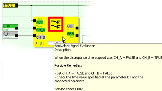
Figure 2-8 Example of an online tool tip in the event of an error
