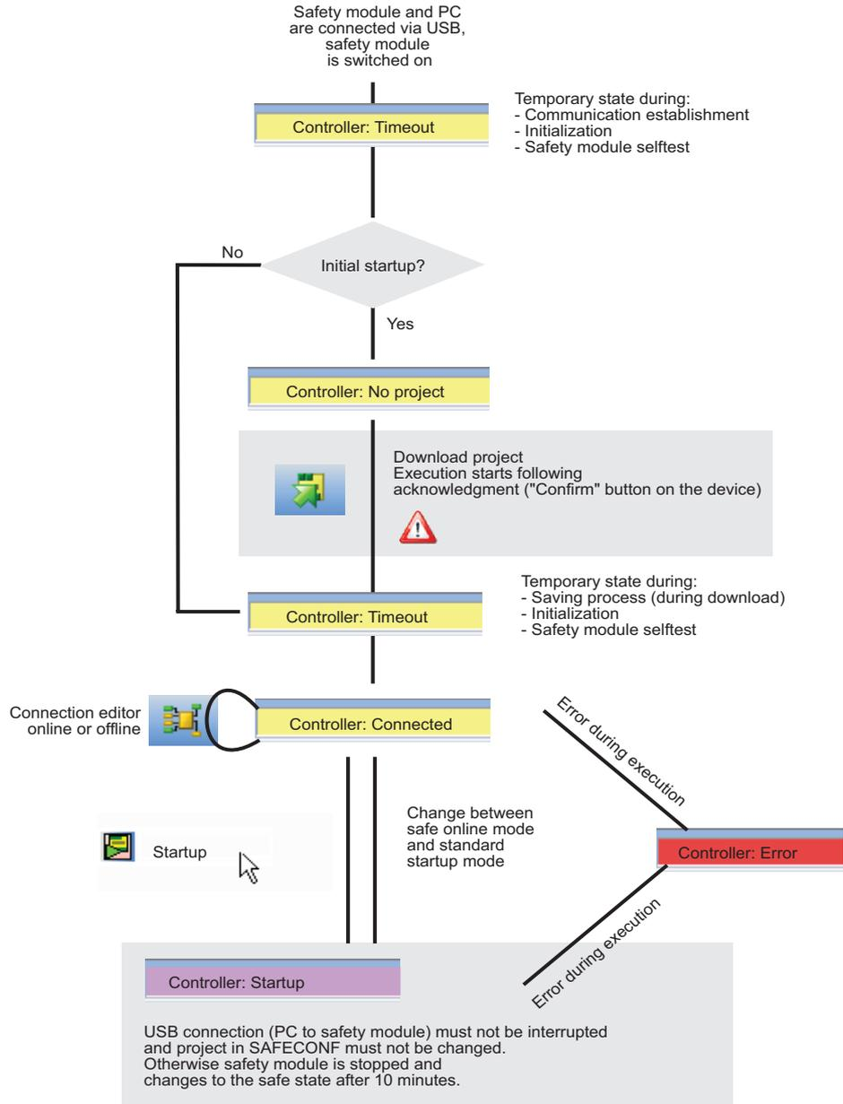
Figure 3-3 Diagram: Possible operating modes (status) for the PSR-TRISAFE-S safety module
