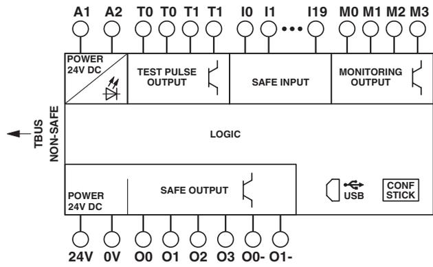
Figure 3-2 Block diagram for the PSR-TRISAFE-S safety module
