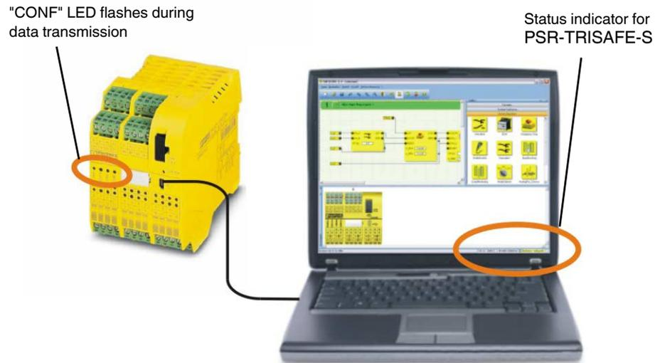
Figure 5-4 USB connection between PC and safety module
