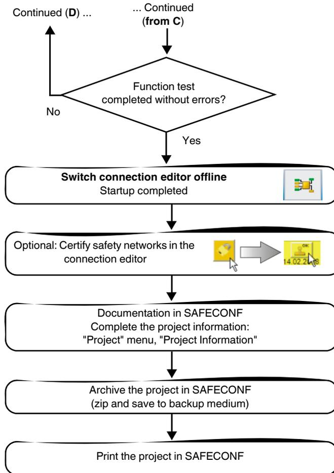
Figure 5-3 Flowchart: Configuration from A to Z (3 of 3)
