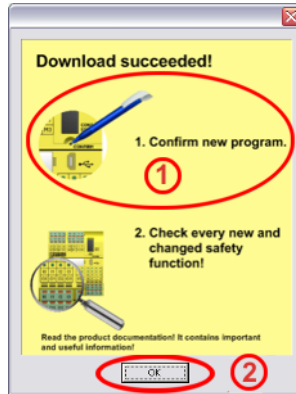
Figure 5-5 Message dialog box following successful data transmission
