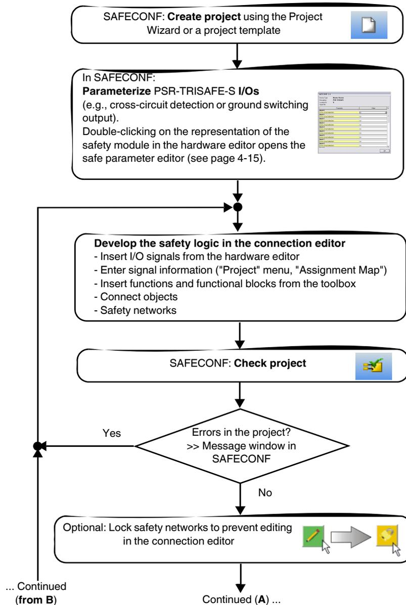
Figure 5-1 Flowchart: Configuration from A to Z (1 of 3)
