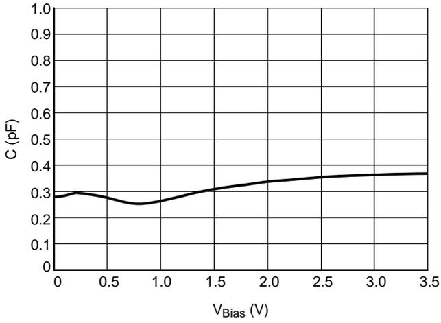
Figure 1. CV Characteristics
