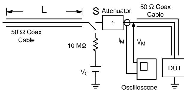
Figure 10. Simplified Schematic of a Typical TLP System
