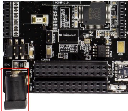
Figure 5. DC Jack connector location
