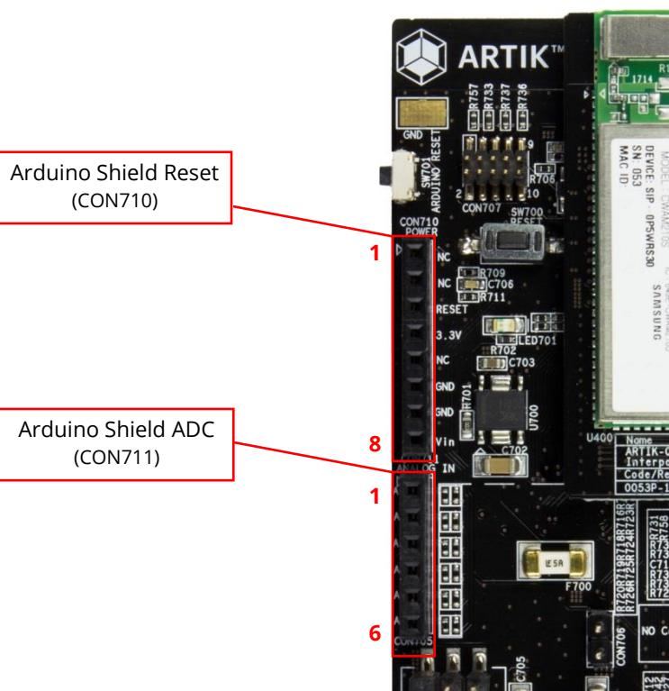
Figure 10. Reset and ADC connector location
