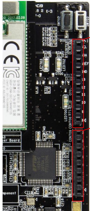
\* Arduino Shield functionality - ARTIK 053 functionality.
