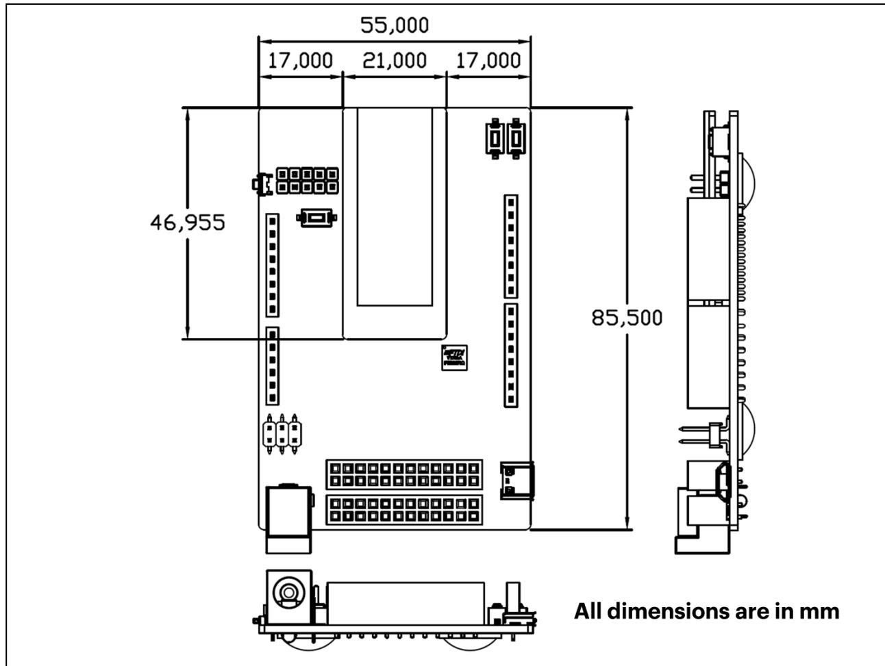
Figure 15. Mechanical Dimensions ARTIK 053 Starter Kit
