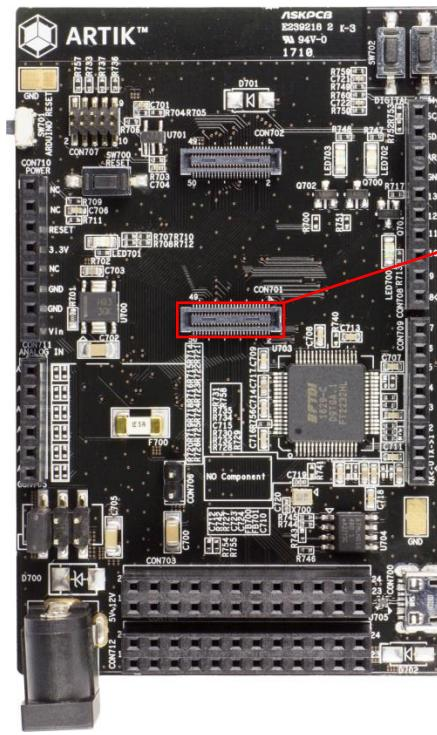
Figure 17. Interposer connector location
