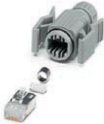
RJ45 sleeve housing, IP67, with push-pull interlocking for panel mounting frames, for cable cross section 5.0 mm ... 6.5 mm, with pin insert VS-08-ST-RJ45, CAT5e, for litz wires AWG 26 and solid wires AWG 26 ... 24
