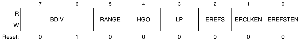
Figure 10-4. ICS Control Register 2 (ICSC2)
