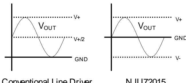
Fig.2 Capacitor-free Operation
