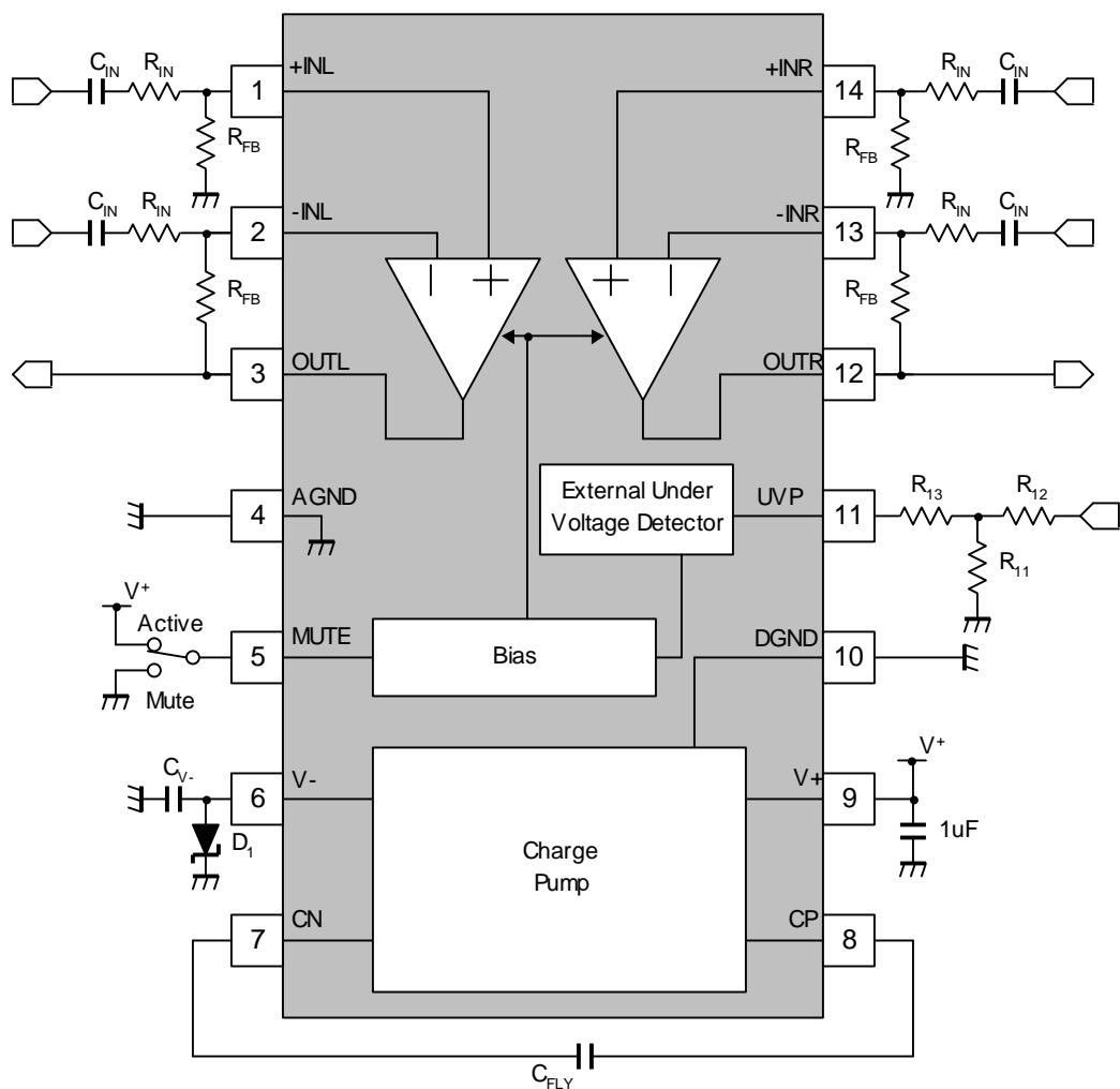
\*1) Connect a zener diode between V- terminal[6pin] and GND terminal[8pin] to prevent connecting V- terminal[6pin] and V+ terminal[3pin].
