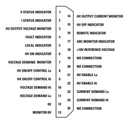
All logical indicators are open collector outputs rated at 16V (max) in the off state. An internal  $100\Omega$  resistor is connected in series with the open collector transistor. The pull down voltage is 0.9V plus the internal resistor drop.
