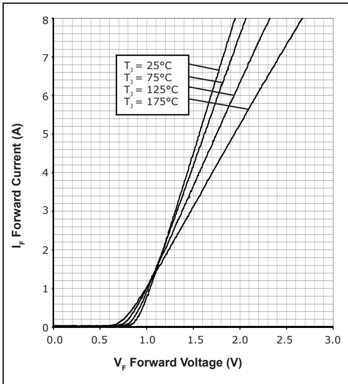
Figure 1. Forward Characteristics
