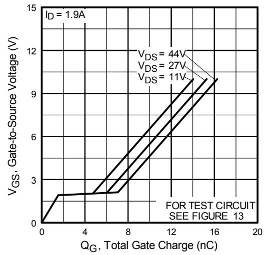
**Fig 6.** Typical Gate Charge vs.
