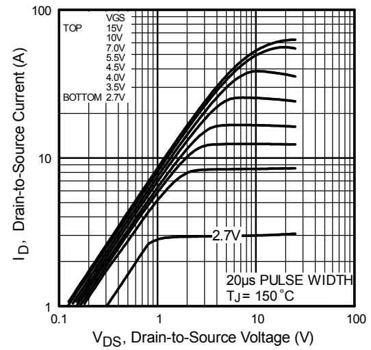
**Fig. 2** Typical Output Characteristics
