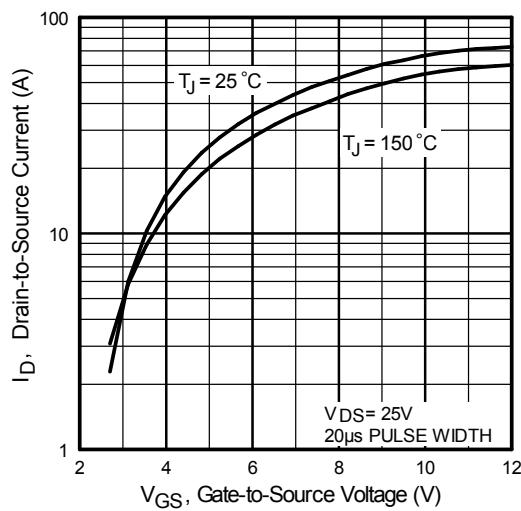
**Fig. 3** Typical Transfer Characteristics
