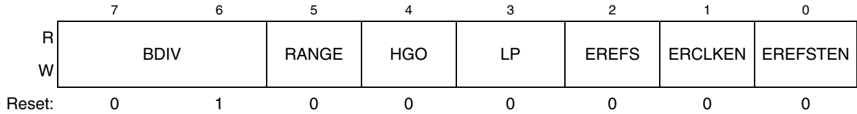
Figure 12-4. MCG Control Register 2 (MCGC2)
