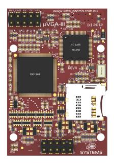
Audio support provided on the display module is supplied by the **PICASO** processor, outputting a line-level audio signal, ready to drive an external amplifier of choice. A simple instruction enables the user to play audio files while continuing the execution of the user application code, such as display updates, communications and much more.
