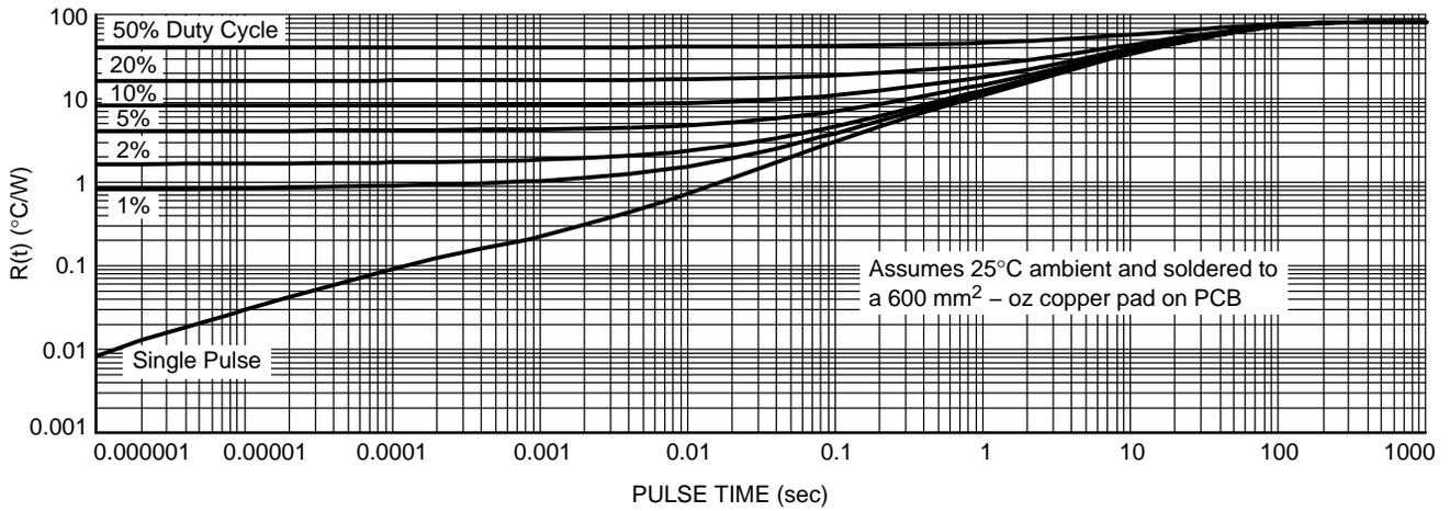
Figure 8. Thermal Characteristics
