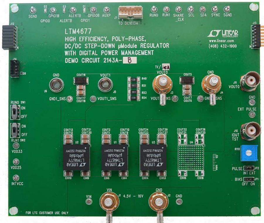
Figure 1. 3x LTM4677; 108A DC2143A-B Demo Circuit
