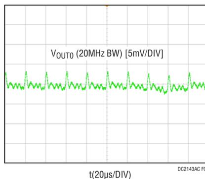
Figure 7. Output Voltage Ripple at  $V_{IN} = 12V$ ,  $V_{OUT} = 1V$ ,  $I_{OUT} = 108A$ ,  $f_{SW} = 500kHz$
