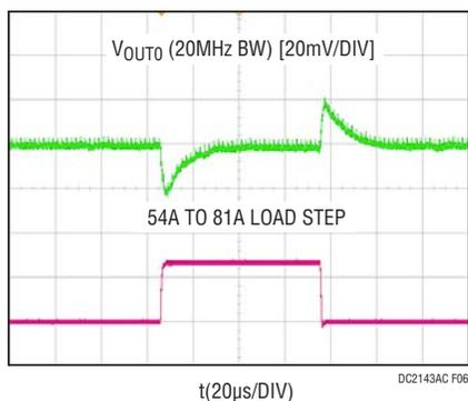
Figure 6. Output Voltage  $V_{OUT}$  vs Load Current at  $V_{IN} = 12V$ ,  $V_{OUT} = 1V$ ,  $f_{SW} = 500kHz$
