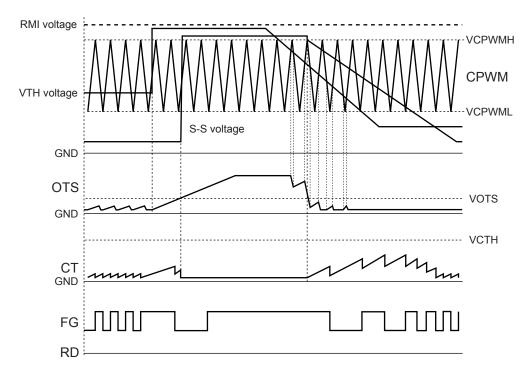
When the output duty ratio based on the VTH/RMI input drops to below 1% or so, the OTS voltage rises, and when it reaches VOTS, the standby mode is established, the CT pin discharges, and the S-S pin is charged. In the standby mode, if the drive mode has been established again by the VTH/RMI input, the rotation is started immediately with soft start. The CT pin discharges at the same time as the switching of FG. For details on lock protection, refer to (2).
