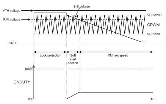
Adjust the S-S pin voltage gradient by means of the capacitance of the capacitor between the S-S pin and REG. Recommended capacitor:  $0.1\mu$  to  $1\mu$ F
