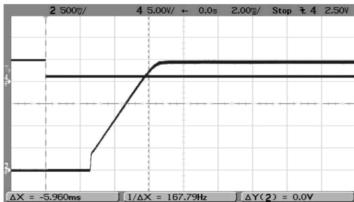
Step Load Transient Response (Vin=12V, Vout=2.5V, Clod=0, Iout=1.5A to 3A) Trace 2=Vout, 100 mV/div. Trace 4=Iout, 2.5A/div.
