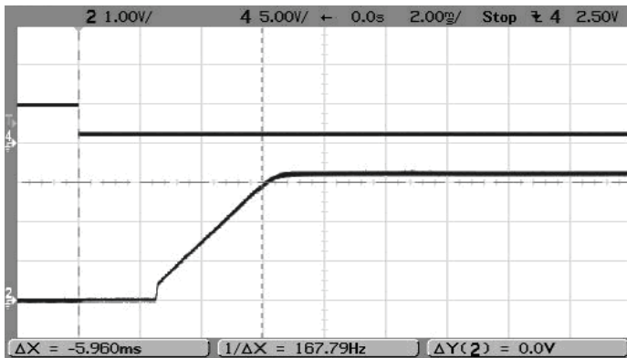
On/Off Enable Startup Delay (Vin=12V, Vout=3.3V, Iout=3A, Cload=0) Trace 4=Enable In, Trace2=Vout
