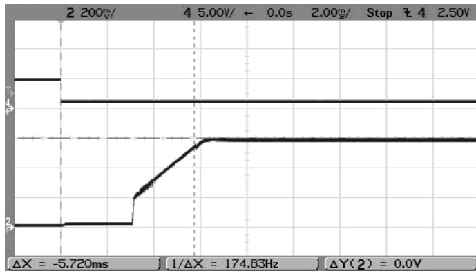
On/Off Enable Startup Delay (Vin=12V, Vout=0.591V, Iout=3A, Cload=0) Trace 4=Enable In, Trace2=Vout
