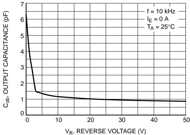
Figure 19. Output Capacitance
