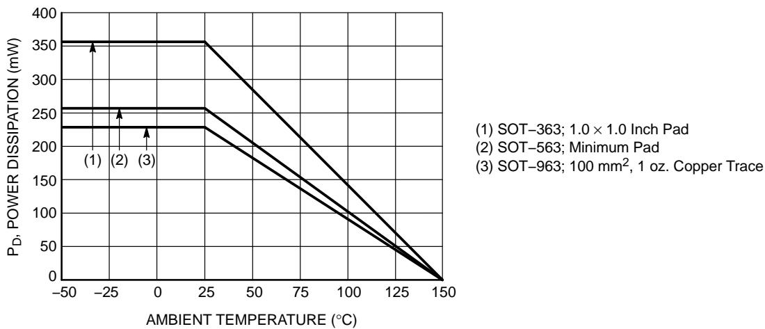
Figure 1. Derating Curve
