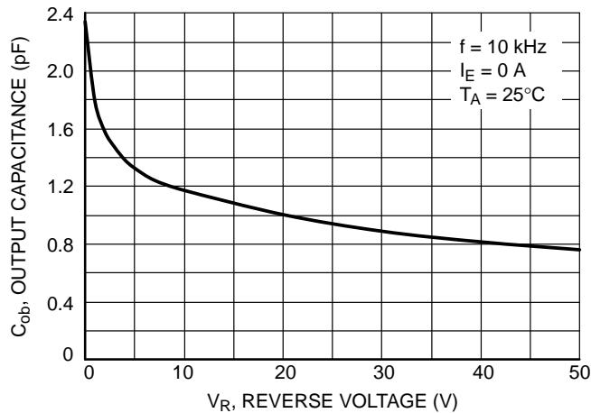
Figure 14. Output Capacitance
