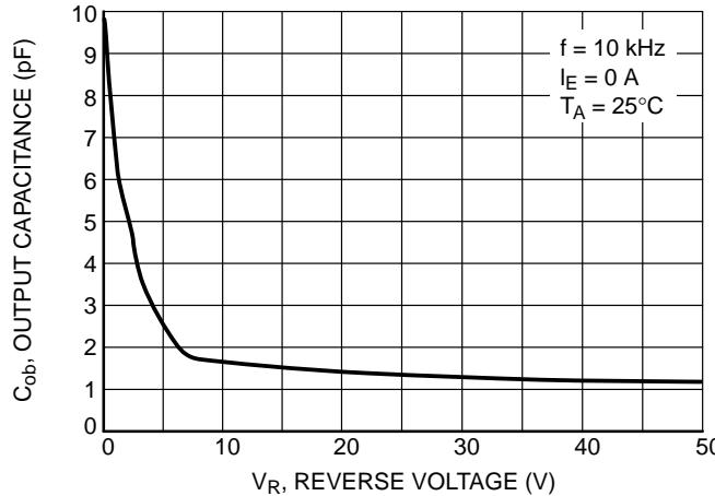
Figure 9. Output Capacitance
